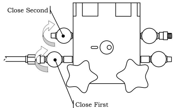
**Step 12:** Close the check valve on the flow meter by turning anti-clockwise.
