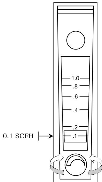
**Step 6:** Close the check valve on the flow meter by turning anti-clockwise.
