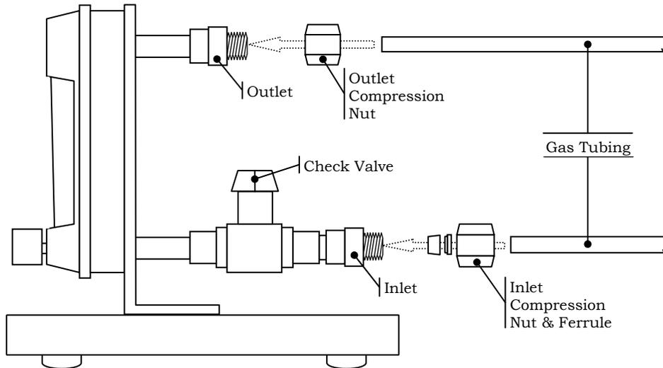
**Step 2:** Ensure that the main valve on the gas cylinder is closed at this time and that the appropriate 2-stage gas regulator is firmly attached to the tank. Connect tubing from the flow meter inlet to the regulator. Use gas-tight compression fittings (tubing and fittings for regulator connection are not included).
