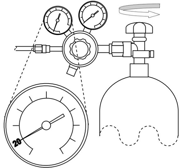
**Step 5:** Set the flow rate to 0.1 SCFH (0.05 LPM) by rotating the adjustment knob either clockwise or anti-clockwise.
