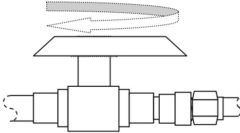
**Step 4:** Open the main valve on the gas cylinder to begin the flow of gas. Set the regulator pressure to 20 psig (140 kpag).
