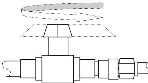
**Step 13:** Close the main valve on the gas cylinder.
