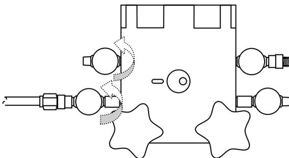
**Step 9:** To begin the flow of gas through the permeation chamber, open the check valve on the flow meter by turning clockwise.
