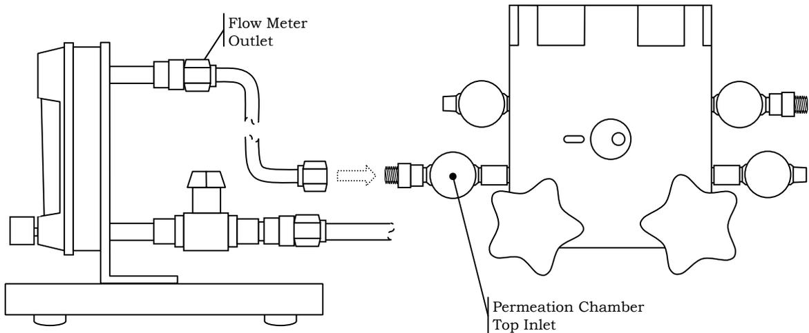
**Step 8:** Fully open both the inlet and outlet valves on the permeation chamber by turning the valves anti-clockwise.
